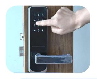
When you enter the unlock password, you can enter the anti-peeping password before and after the correct password. for better privacy.
